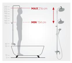
refers to the installation of the mixer at a height of 60 cm from floor level and a bathtub installed 10 cm above floor level.
