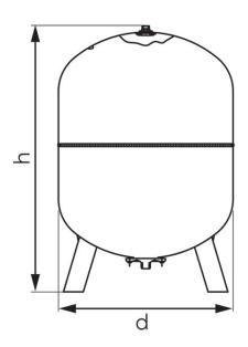
max. working pressure: 10 barprecharge pressure: 3.5 bar
