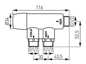
• maximal water temperature: 90°C
