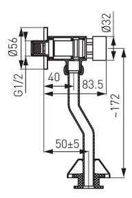
The Z211 urinal valve based on PN-EN 12541: 2005 classified as a 1.5-liter valve, which means that the valve is destined to supply 1.5 litres of water. It is the most economical of the class in the urinal valve norm.
